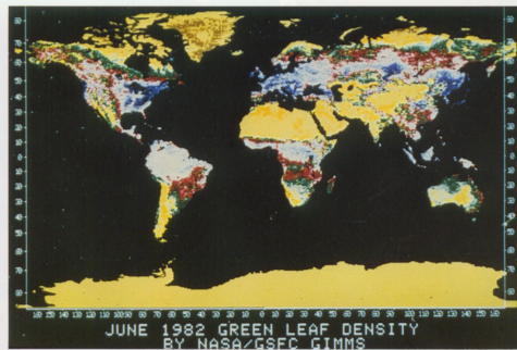
Plate 1 Normalized Difference Vegetation Index (NDVI) for June 1982 as obtained from the Advanced Very High Resolution Radiometer on the NOAA satellite. Note that the greatest vegetation density is colored white and blue, whereas green and yellow indicate lower leaf area. The Northern Hemisphere is in mid-summer. From NASA, 1987, Moderate-Resolution Imaging Spectrometer, Instrument Report, Washington D.C.
