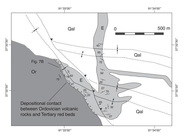
Figure 9. Detailed geologic map showing the unconformity between Paleogene strata (E) and Ordovician metavolcanics (Or). The area is mostly covered by Quaternary alluvial and loess deposits (Qal), except the deep-cut gullies. Note that the Cenozoic strata themselves are folded and cut by south-directed thrusts.
