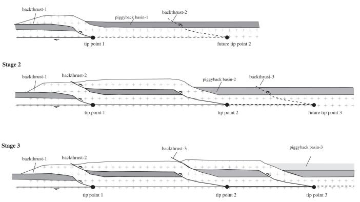
Figure 14. A piece-meal accretion model for the uplift history of the Qimen Tagh Mountains and the development of the south-directed Qimen Tagh–Yousha Shan thrust belt. In this model, a large piggyback basin was first developed on the backlimb of a large backthrust that had climbed up the range front. The piggyback basin was subsequently fragmented by younger backthrusts developed to the north in the foreland as a result of northward propagation of a wedge tip.
