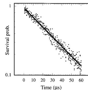
**Figure 2** Typical example of experimentally measured survival probability for a small acceleration of  $1,200 \text{ m s}^{-2}$ , a large acceleration of  $4,500 \text{ m s}^{-2}$ , and  $V_0/\hbar = 50$  kHz as a function of the duration of the large acceleration. Note that the vertical axis is logarithmic. The solid line is a fit to an exponential.
