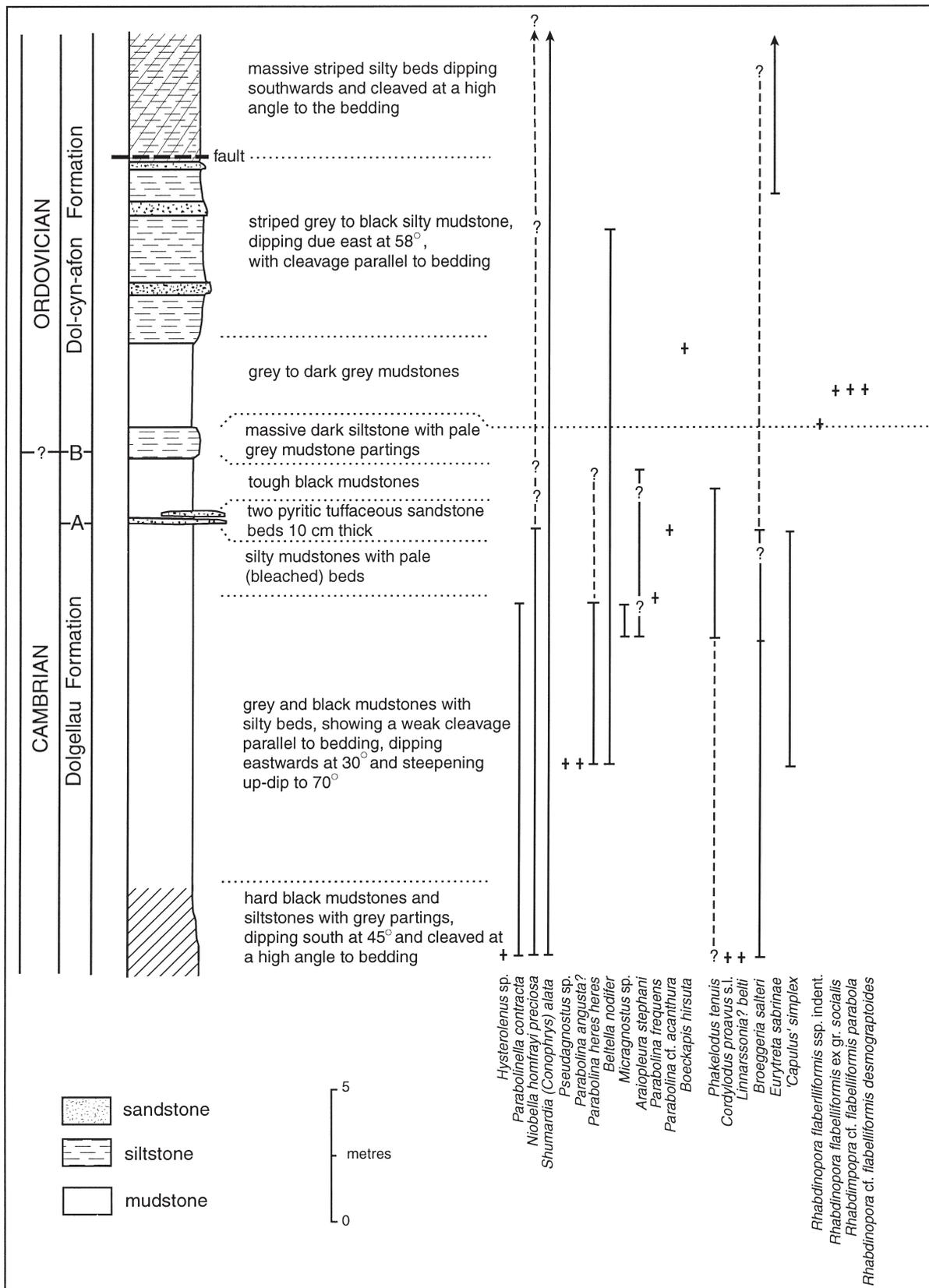
Figure 2. Cambrian–Ordovician boundary interval on Bryn-llin-fawr road, after Rushton *et al.* (2000). Faunal distribution updated from Rushton (1982). Alternative definitions of base of Dol-cyn-afon Formation from change to lighter-coloured siltstones (at B) (Rushton, 1982, upper boundary) or at sequence boundary defined by lower feldspathic sandstone (A, this report, lower contact). Diagonal ruling in lithological column emphasizes presence of slaty cleavage at high angle to bedding.
