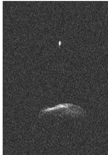
Figure 1: Range-Doppler image showing the two components of 2000 DP107. It was obtained in September 2008 and has a range resolution of 30 m.
