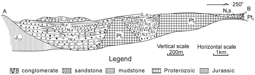
FIG. 8. Profile across the South Xorkol Area, showing characteristics of a typical channel filling series. The vertical scale is 6x the horizontal scale in order to show the texture inside the basin more clearly. See Figure 7 and the map legend for explanation. Legend: Q<sub>1-2</sub> = Lower-Middle Pleistocene Qigequan Formation; N<sub>2s</sub> = Pliocene Shizigou Formation; J<sub>2-3</sub> = Middle-Upper Jurassic; Pt<sub>2</sub> = Proterozoic.
