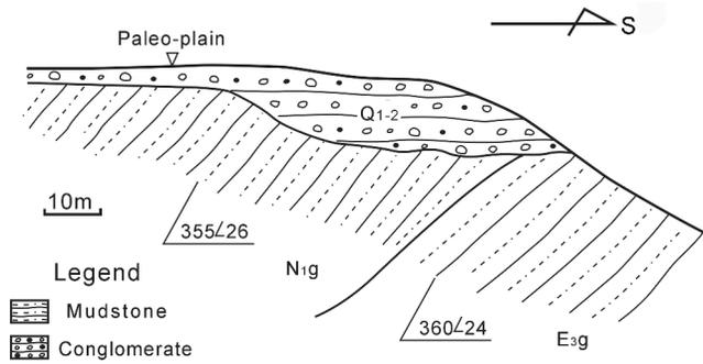
FIG. 4. Unconformity contact between the Lower Quaternary conglomerate and the Tertiary mudstone. Legend: E<sub>3g</sub> = Oligocene Xia Ganchaigou Formation; N<sub>1g</sub> = Miocene Shang Ganchaigou Formation; Q<sub>1-2</sub> = Lower–Middle Pleistocene Qigequan Formation.
