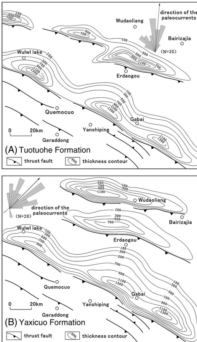
**Fig. 8.** Sedimentary rock isopach map (in meters) and paleocurrents of the Tuotuohe and Yaxicuo formations (rose plot for unidirectional strikes of paleocurrents, arrow shows mean direction, N = number of data).
