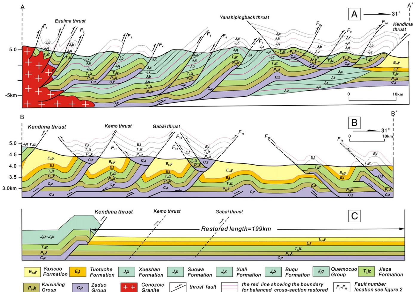
Fig. 3. Cross sections of the Tanggula thrust system (A) and Tuotuohe Basin (B), showing the deformation of TTS and syncontractural basin development associated with Paleocene–Oligocene shortening. Restored cross-section of A–A' (C).
