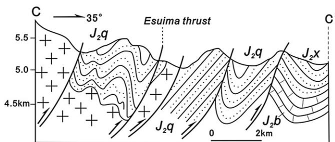
**Fig. 6.** Cross section of root thrust zone in the Esuima area, location and legend seeing Figs. 2 and 3.
