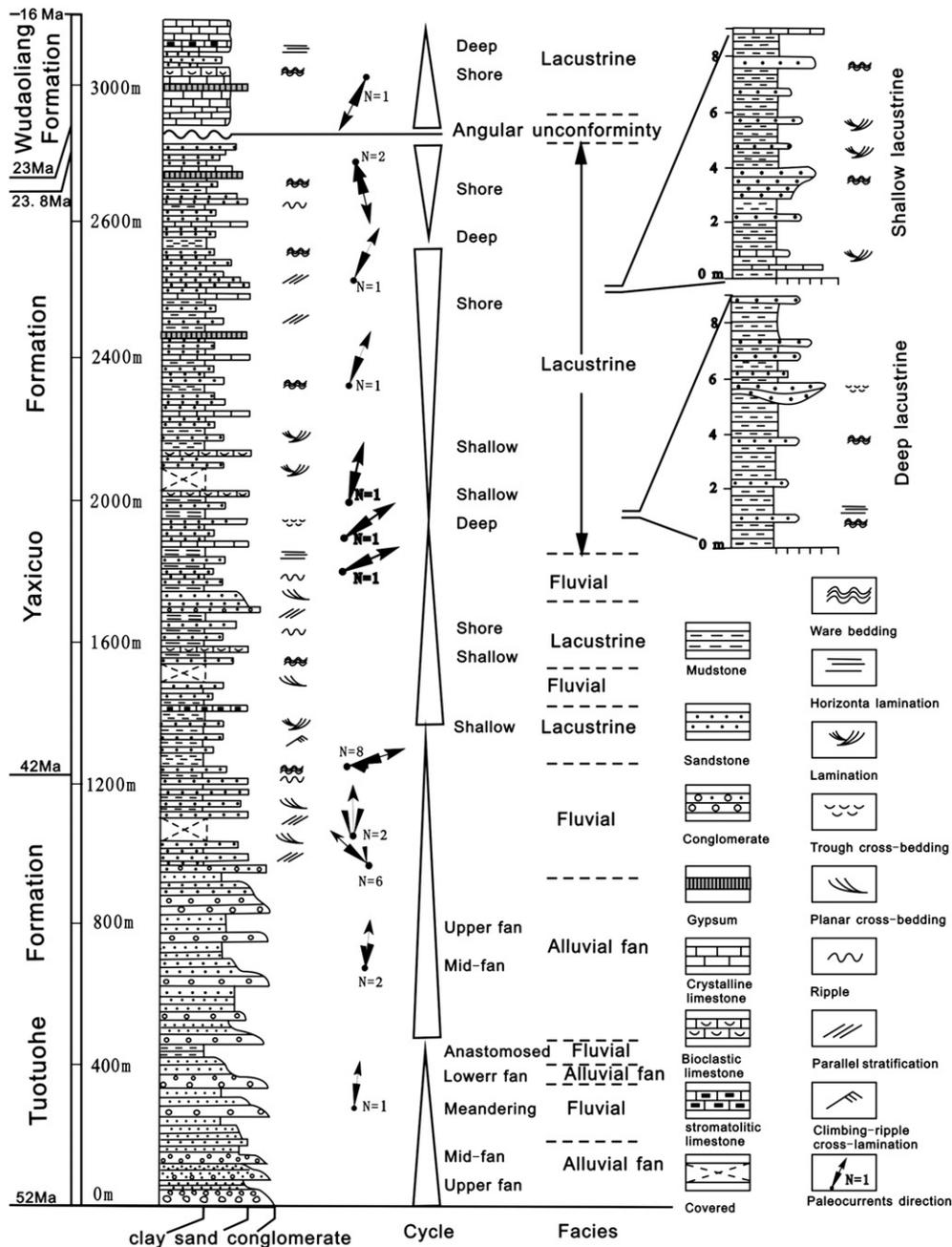
Fig. 7. Logs of the Tertiary strata in the Tuotuohe Basin. See Fig. 2 for location of measured section.
