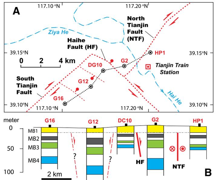
Figure 4. A: Simplified active fault map of the Tianjin area (north China) modified from Chen et al. (2004). B: Simplified stratigraphic sections revealed by a series of drill cores (shown as black dots inside black circles; drill-core numbers are labeled in red) across the Tangshan-Hejian-Cixian fault zone in the Tianjin area. Data are from Chen et al. (2004).
